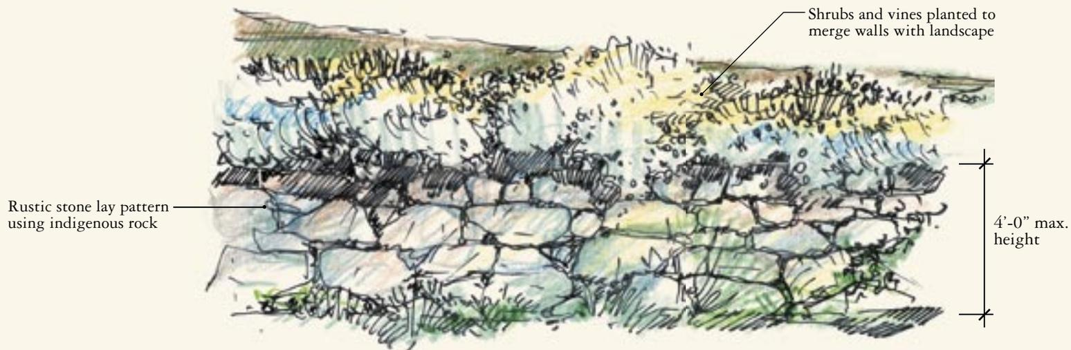
FIGURE 2.1: Retaining wall design
